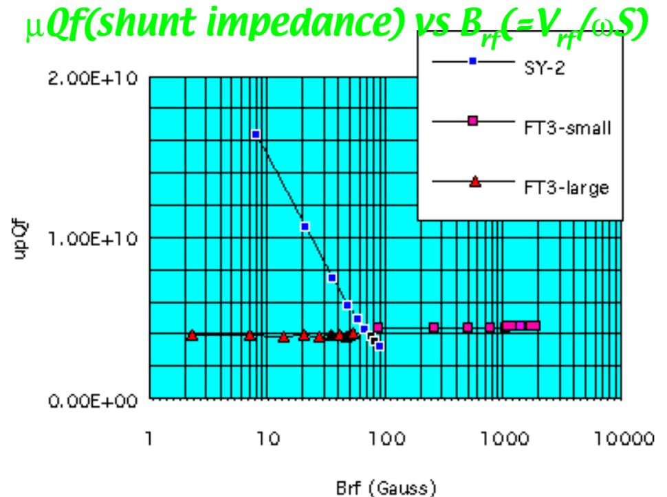
Typical characteristics of Ni-Zn ferrite and Magnetic Alloy(FINEMET).
