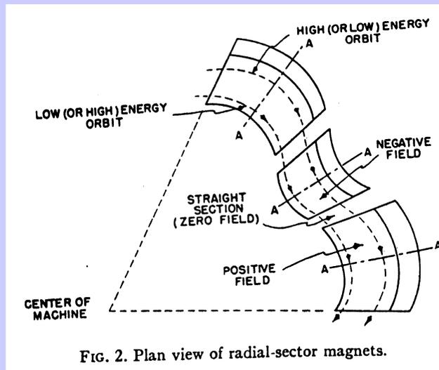
FIG. 2. Plan view of radial-sector magnets.
