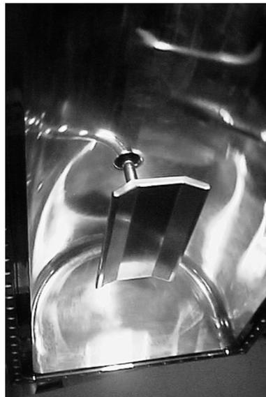
**Fig. 55:** High-energy (HE) piston tuner inside the tank
